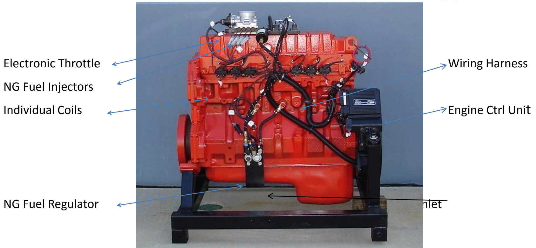
REPOWER: MY 2011 esi0308 7.6 L CNG Engine 280hp, 860 lb-ft torque
