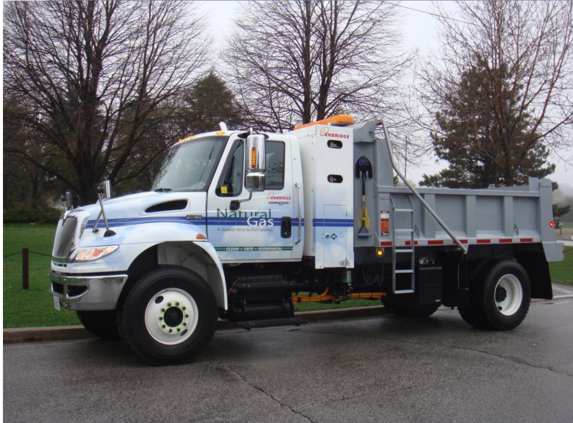
ENBRIDGE GAS, Toronto, Canada, MY 2010 International Truck 4300 series Powered My 2010 ESI Phoenix NG 7.6 L dedicated CNG engine
