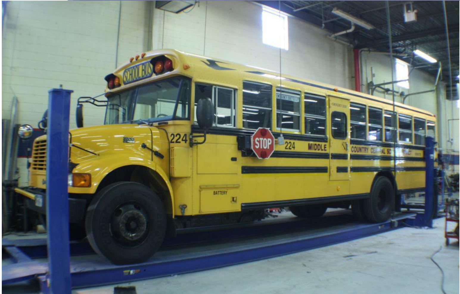
MY 2000 IC Bus Chassis with DT466E (6 units) Powered by MY2010 ESI 7.6 Liter dedicated CNG Engine
