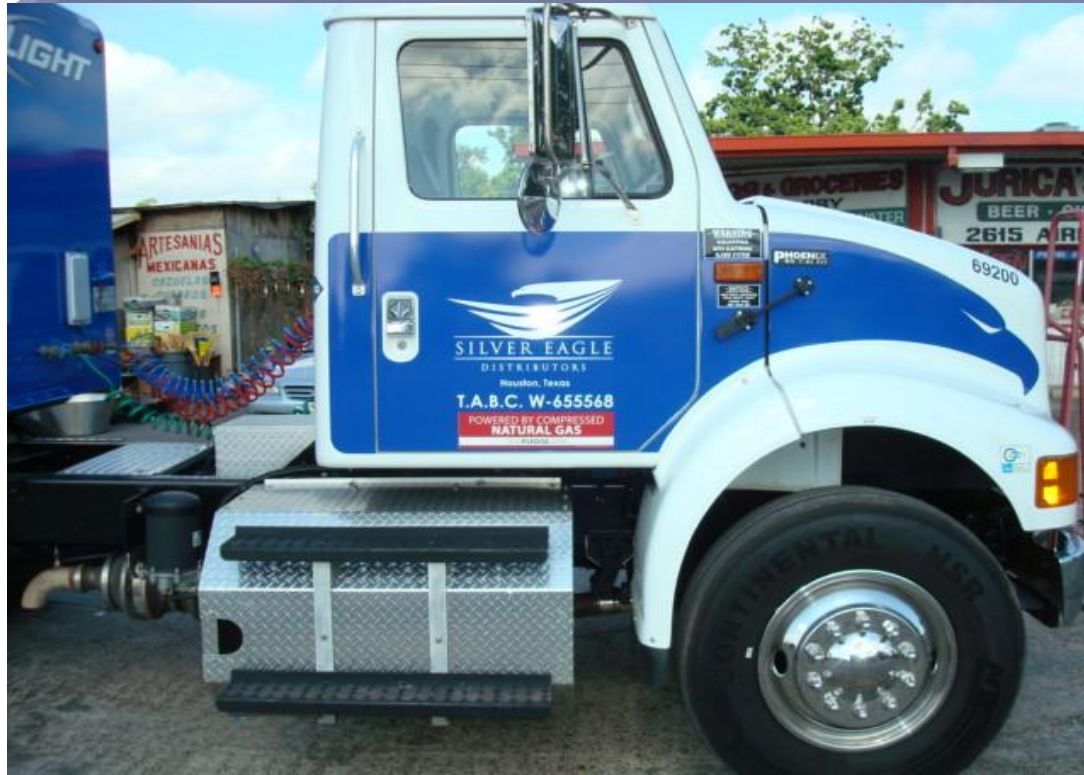
Silver Eagle Distributors LLP - Houston World's largest AB Distributor MY1999 Tractor Powered by MY2006 ESI 7.6 L CNG Engine
