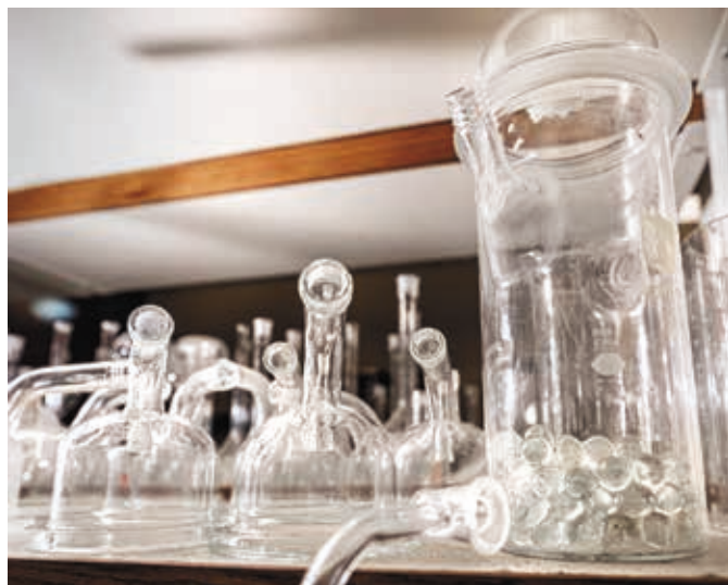
Researchers in this lab at LSU have developed custom microbial habitats, or bioreactors, that are used to break down dangerous pollutants in the environment.
